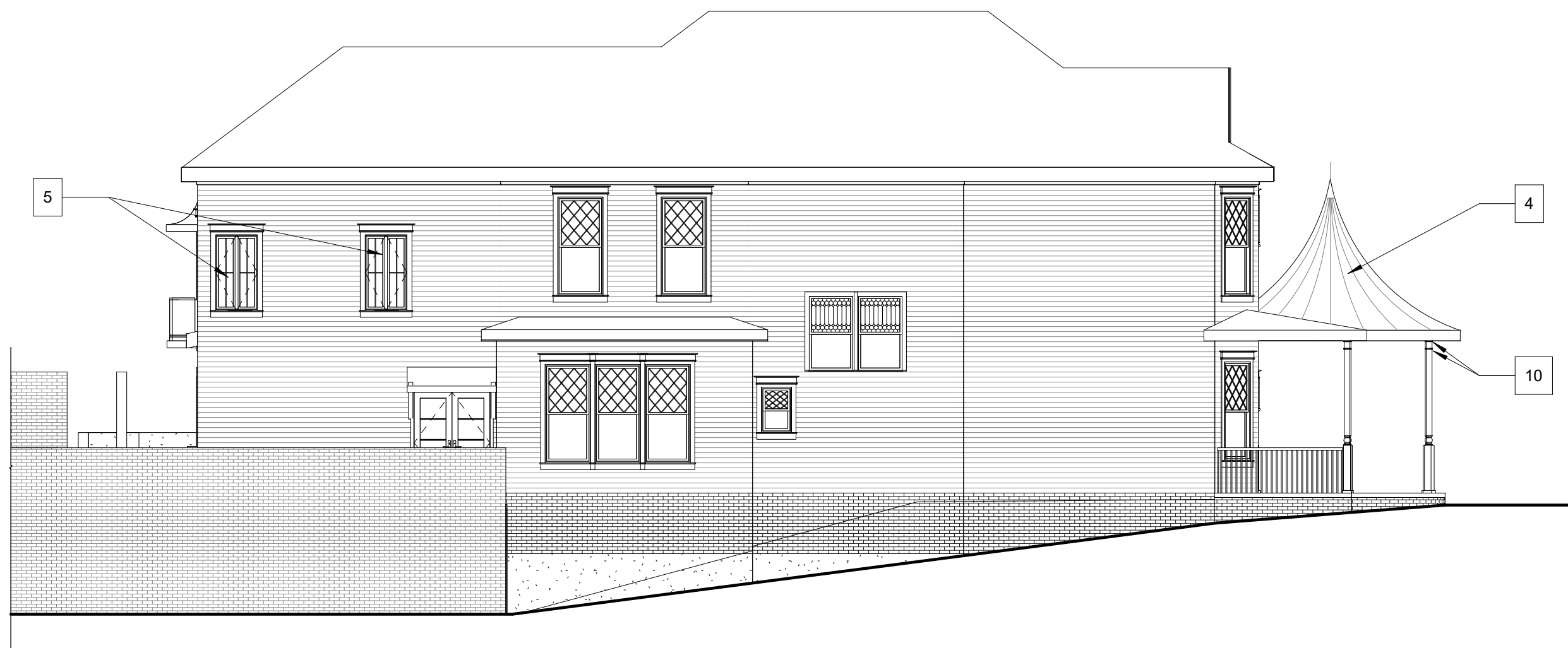
7 PROPOSED SIDE ELEVATION - NE PR.1 1/8" = 1'-0"
