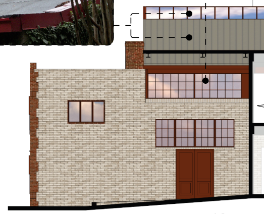
SIDE ELEVATION: WINDOW INFILL (STYLE), RAISE GABLE ROOF UP 5'-8" - MAINTAINING SKYLIGHTS & TRUSSES, NEW WINDOWS (STYLE)
