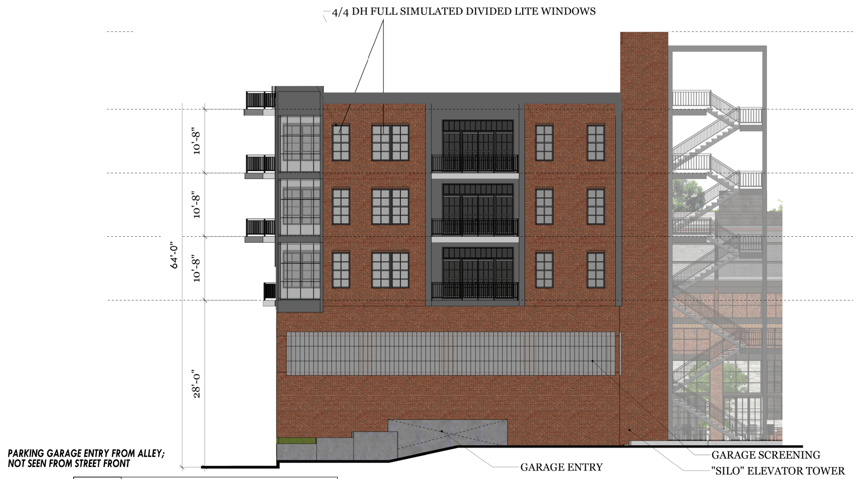
A,1 BLDG C - WEST ELEVATION 1/8" = 1'-0" 1/16" = 1'-0" WHEN PRINTED AT HALF SCALE ON 11x17
